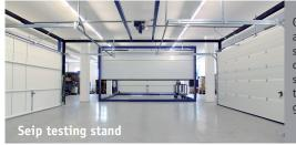
Our door operators are being tested for safety standards in our factory testing stands with different types and sizes of garage doors.
